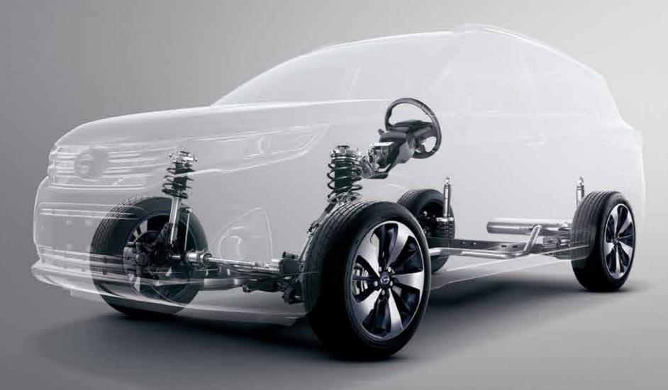
• McPherson independent front suspension and torsion beam rear suspension A perfect balance between road condition feedback and driving comfort.
